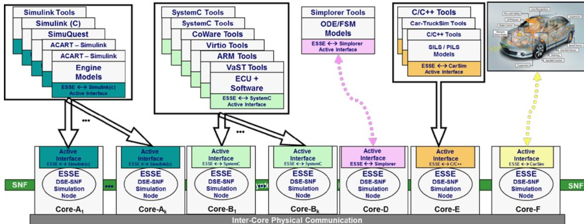
EST has solved this problem by inventing the world’s highest performing scalable, multi-core, distributed simulation engine (DSE). The ESSE DSE is depicted above supporting many models, simulators and tools from many sources and with varying levels of fidelity in function and timing.
